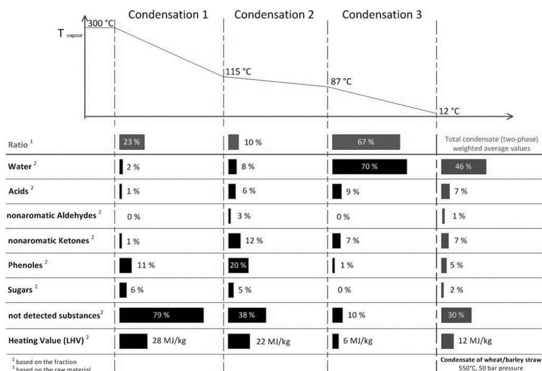
Figure 3. Lumped composition of liquids collected from three stage condensation.
