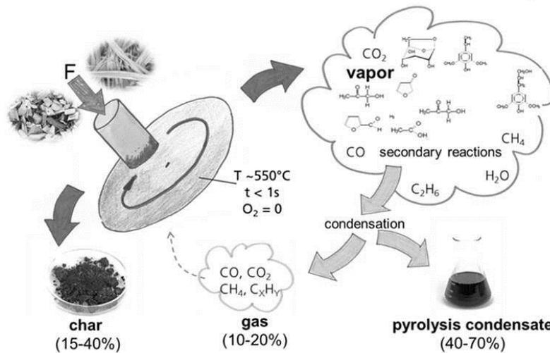
Figure 1. Schematic diagram of fast pyrolysis principle
