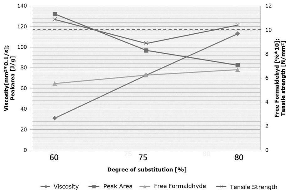
Figure 4. Variation of characteristic properties of phenol-formaldehyde resins over degree of substitution.
