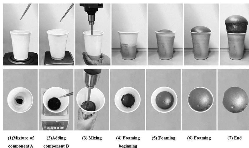
Figure 5. Production process of polyurethane foam samples with pyrolysis condensates.
