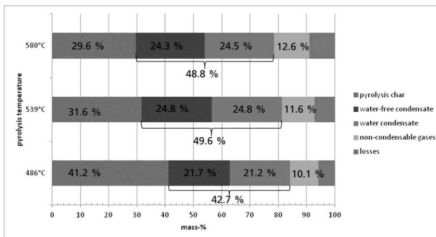
Figure 2. Mass balance of fast pyrolysis of straw at different pyrolysis temperatures
