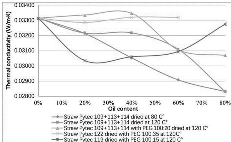
Figure 6. Thermal conductivity of polyurethane foams produced with straw-based pyrolysis condensates.
