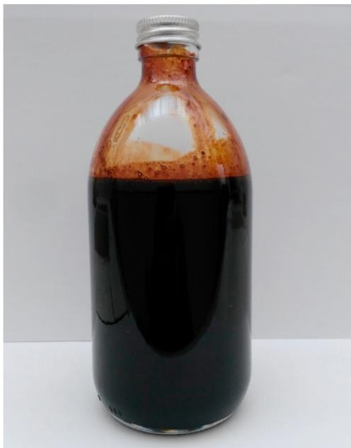
**Picture 1.** Ablative flash pyrolysis bio-oil from lignocellulosic biomass.
