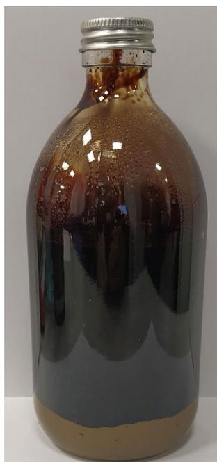
**Figure 2:** Two -phase product from bio-oil hydrotreatment of RUN-03
