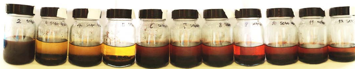
Figure 7: Catalytically upgraded (activated carbon catalyst A) straw-based bio-oil (total condensates)
