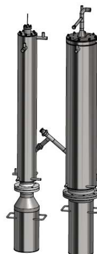
Figure 4: 1 st stage condensation step (condenser on the right and ESP on the left side)
